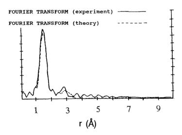
Fig. 2. EXAFS and Fourier transforms for solid MnO<sub>3</sub>F.
